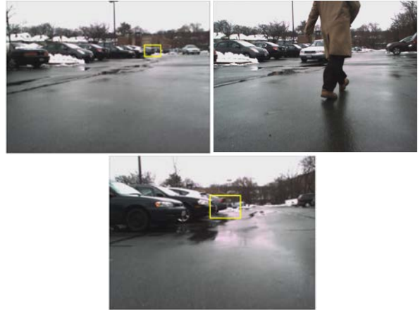
Figure 7: Occlusion handling during point-and-go navigation. The system is capable of re-acquiring an initially selected goal despite multiple occlusions by moving objects and change in perspective.
