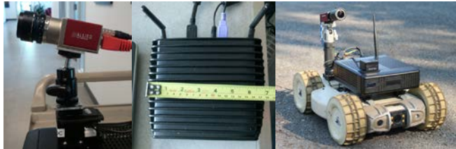
Figure 2: Vision-based autonomy appliqué components, consisting of an Allied Vision Technology Mako camera and Dynamixel servo (left), and a compact, fanless IntensePC computer (center). System installed on a Dragon Runner SUGV (right).
